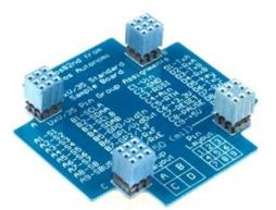
This is a UxV/35 standard pinout definition on a UxV/35 board. The pin numbering, pin grouping and pin assignments are clearly shown.
