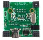
The Serial Test board provides two USB serial ports that can be routed to any of the serial signals that are used on the UxV/35 bus. Solder Jumpers on the back of the board help select the Tx/Rx polarity and what port is mapped to either of the USB serial channels. This board can also be used to power the UxV/35 stack from a USB port on a PC for testing and development.
