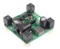
The Power Supply board is used to provide power to the UxV/35 Stack on the bench for development or testing. It provides all three voltages and can be used for UxV/35 simulation as well. The external power input for the board becomes the Vin voltage.
