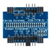
The Serial Loopback board provides a convenient way to loopback any of the serial ports upon themselves for testing and assurance of proper serial port operation.
