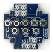
The KeyTest boards allows user testing of each of the inputs on the UxV/35 bus such as Reset, Pause, RTH and all of the General Purpose lines. Led status is also provided for those signals the same way as the Signal Test board with LEDs.
