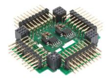
This base board brings out all UxV/35 bus signals in the common 3 pin, .100 inch, servo signal format that is used for servo and serial signals.
