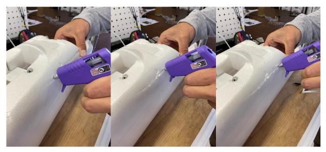
**Step 5:** Clamp and clean up. Use a wetted finger to smooth flat any glue that squeezes out. Apply constant pressure and keep the seam together for at least 2 minutes after gluing.
