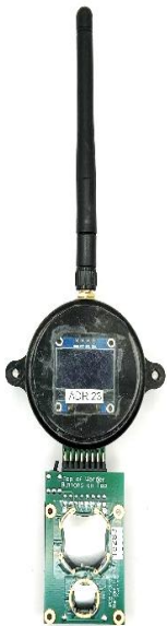
Warden Pilot's safety device. Must send heartbeat and run command in order to operate and run the UAS.
