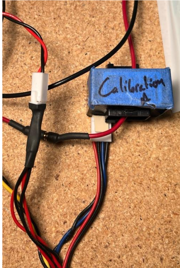
Figure 9: The Tamura current sensor. Show as well is the split for the voltage measurement from the battery.
