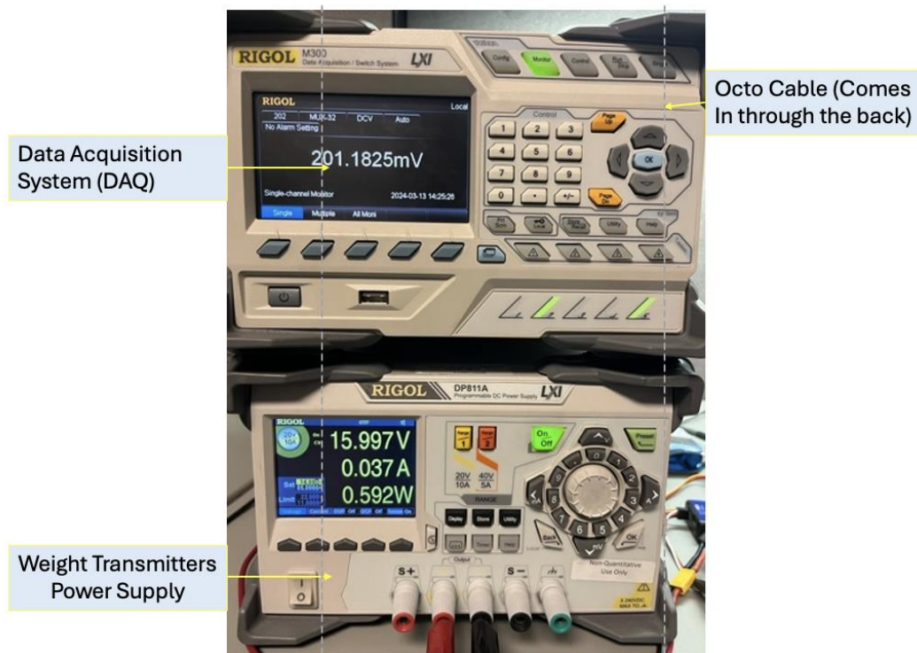
Figure 1: The above is an image of the setup. A shows outside the bird cage B shows inside. Detailed photos are given below labels the many components inside the bird cage. The Octo-Cable comes from inside the bird cage to the outside is meets with the data acquisition system. The Servo control also runs outside the bird cage for safe operation of the motor.
