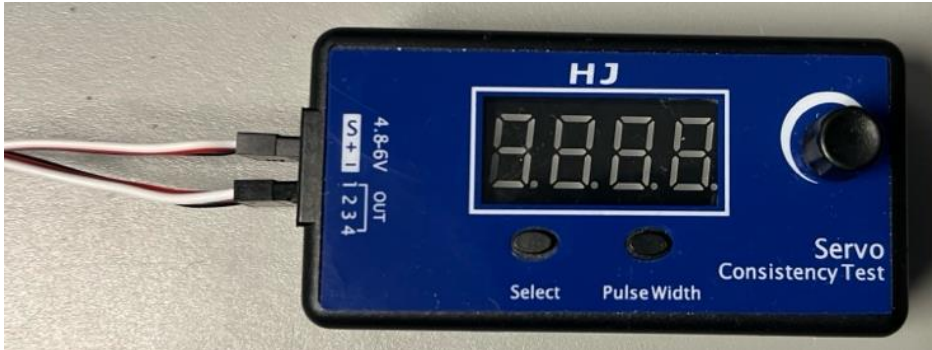
Figure 6: Servo controller used to control the motor set-up.
