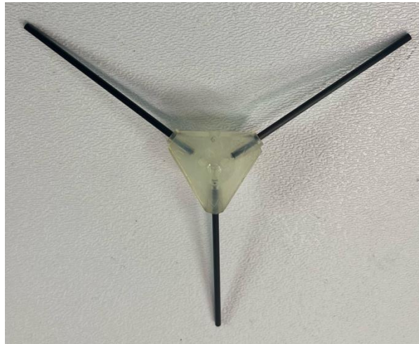
Figure 2: The mold currently used can make larger size flight baskets for larger drones, so long as the edge pieces are strong enough to withstand a crash.
