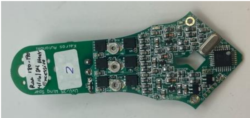
Figure 2: ESC 2. This is paired with a battery base board. Same model as ESC 1.
