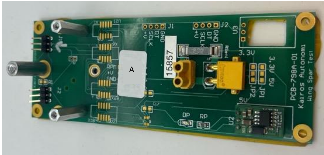
Figure 13: Battery base board A. This model is a little older and was the board used in the testing of different motor and propeller combinations.
