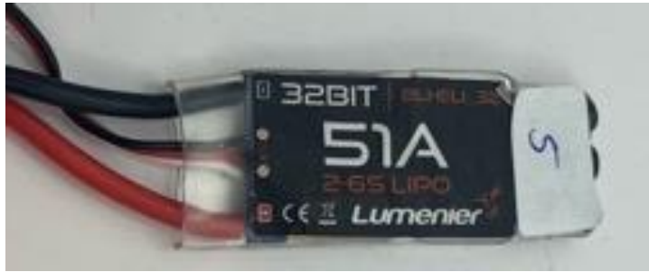
Figure 5: ESC 6. Same Model as ESC 5, without a heat sink.
