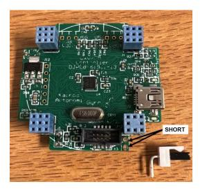
Short a connection between the 2 sockets shown in the picture to the left and ensure a solid connection.
