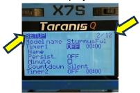
**6)** Spin the **Scroll dial** to scroll down through page 2/12and move the selection reticle (black blinking rectangle) to "[**BND**]" in the row labeled "**RxNum**."
