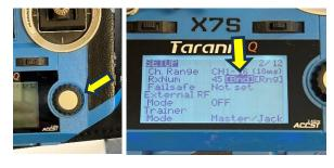
7) Press the **Scroll dial** and a sub-menu will appear. Scroll with the dial to "**Ch9-16 Telem On,**" then press the **Scroll dial** again
