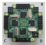
With Kairos assistance, Samtec developed a set of connectors based on a 2mm grid in a 3 x 3 pinning format. Groups A, B, and C use the full 9-pin load. Group D uses an 8-pin load. Without the middle pin, Group D becomes the key.
