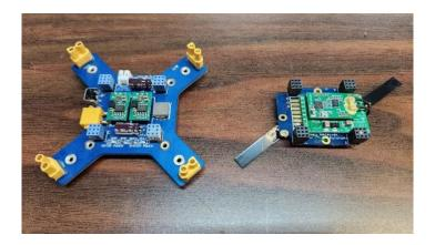
Install the flight radio onto the carrier board after aligning the keyed UxV connectors.
