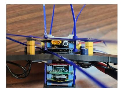
These zip ties are not expected to be very tight. Do not attempt to overly tighten them as this could damage the UxV connectors. The primary purpose of the zip ties and cage are to keep the UxV stack together in aggressive flight and a potential crash. Trim off the excess from all zip ties.
