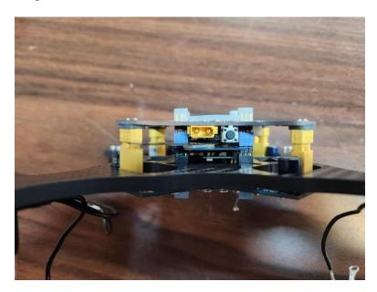
The 4 yellow xt30 connectors should be fully connected when done.
