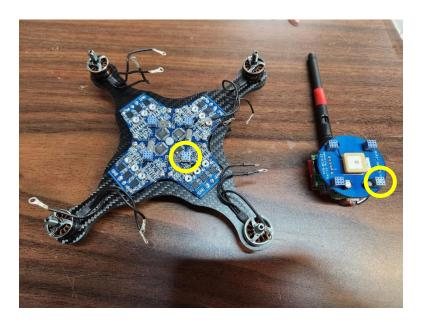
Check that the full stack is connected. Each blue UxV connector should contact the PCB above.
