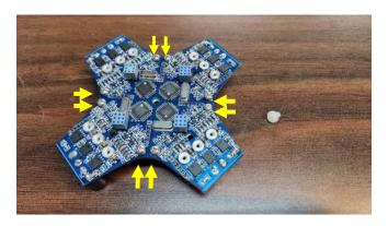
Lastly, install the 6-32" nylon screw into the center location. <u>Do not overtighten this screw as it will easily strip.</u>
