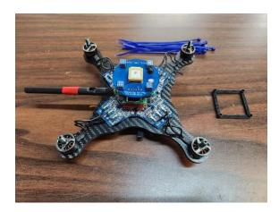
Place the cage on the top of the UxV stack and thread the first zip tie down the stack.
