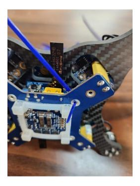
A third zip tie on the bottom of the ESC power carrier board will secure the full stack together. Repeat this step for the 3 remaining corners of the UxV cage.
