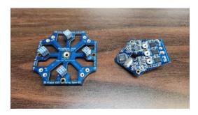
Install the ESC onto the hub in the shown orientation. Carefully press down onto the ESC to prevent damage to the UxV/35 connector.
