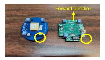
Each UxV board has one keyed connector. These keyed connectors must align when connecting two boards. These keyed connectors also help identify the forward direction as they signify the back right on a UxV/35 drone.
