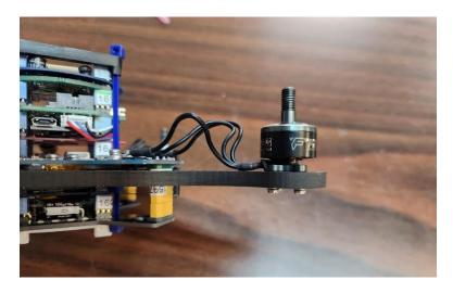
Loose motor wires have the risk of contacting the propeller when flying. Shown above is an example of too much slack in the wires. Tape these down using electrical tape or wrap the motor wires around the frame arm if possible.
