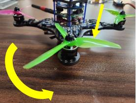
After installing propellers, the drone is ready for a flight test. A drone should always be hand flown in stabilize mode before attempting any missions.
