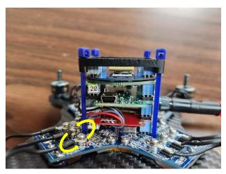
If any motor needs their direction flipped, first <u>power off the drone and disconnect the battery</u>. Then take any two motor wires, remove the screws and swap their locations on the ESC making sure to retighten the screws with a lock washer.
